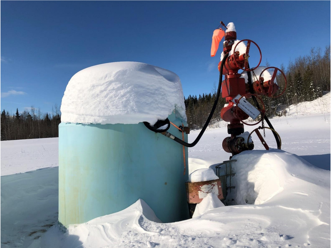
Photo #2: S. Pointed Mountain L-68 well head with SCV connected to tank to collect any liquids.
