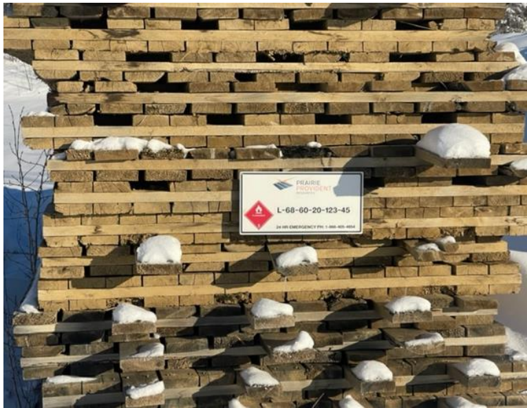
Figure 1 - PPR L-68 Swamp matting / Signage
