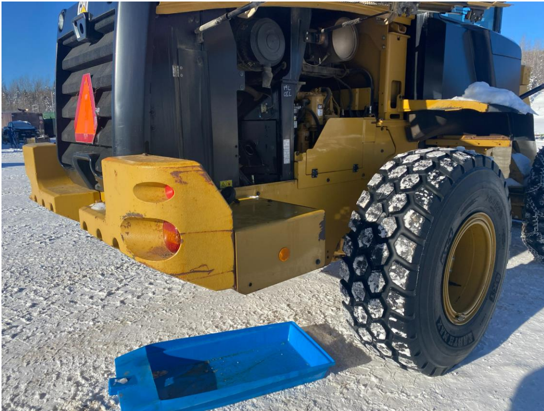
Photo 27: Drip tray under equipment during refueling at tank access port
