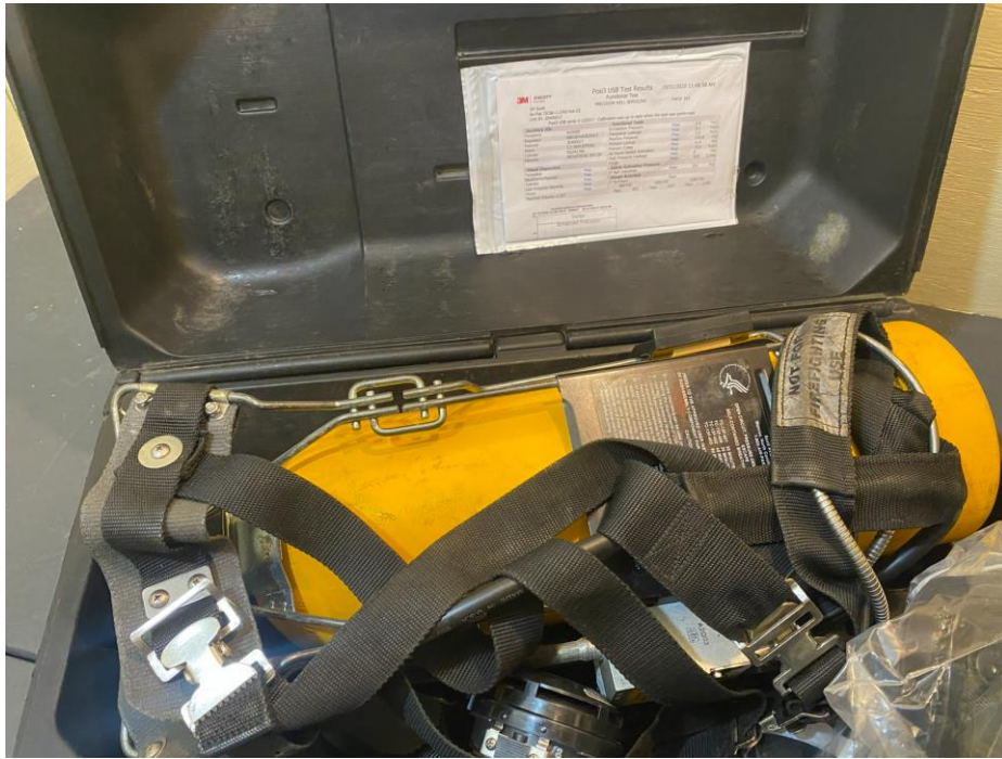
Photo 23: SCBA components inspected and verified with function test documents
