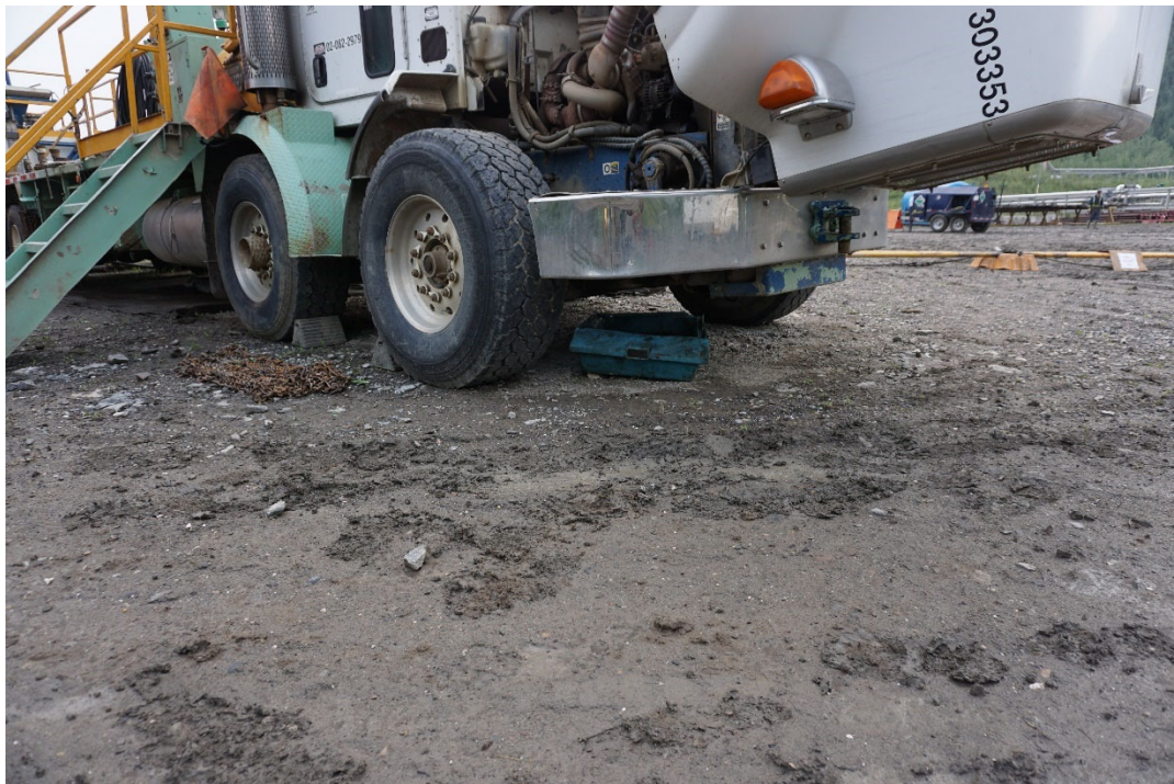
Photo #11: Drip tray placed below parked equipment.
