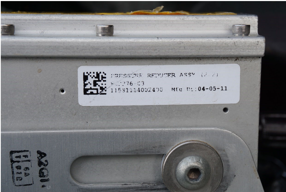
Photo #7: The above noted inspection sheet was assigned to this reducer, but serial numbers did not match.
