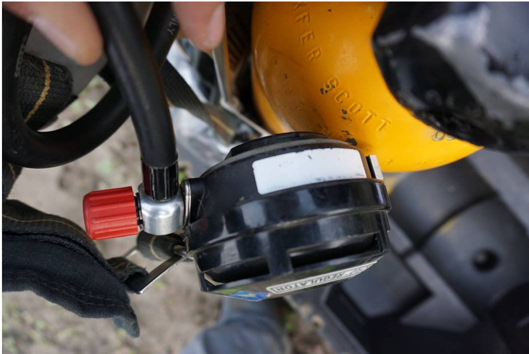
Photo #8: Verification of the SCBA's on site was done through a barcode system however, Serial numbers on United's equipment (reducer/regulator) were not legible or did not match to verify with the Inspection sheet serial numbers. Inspectors recommended replacing the white serial number stickers on the testers equipment so they can be easily confirmed on site during future inspections.
