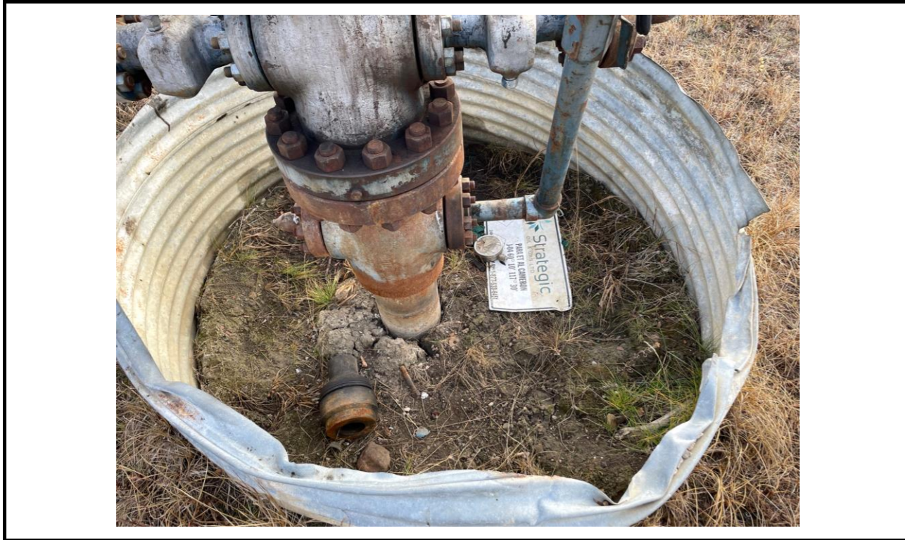
Looking inside cassion with wellhead sign, tubing hanger, and pressure gauge on ground
