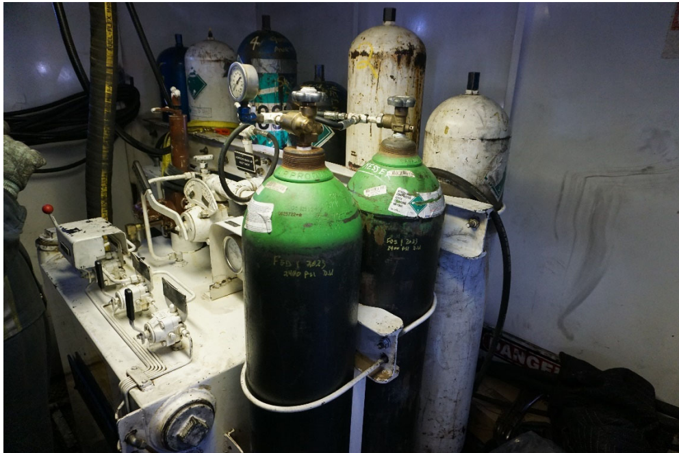
PHOTO #1: View of the Accumulator shack. 6x 11gal Nitrogen tanks with 2x back up tanks.
