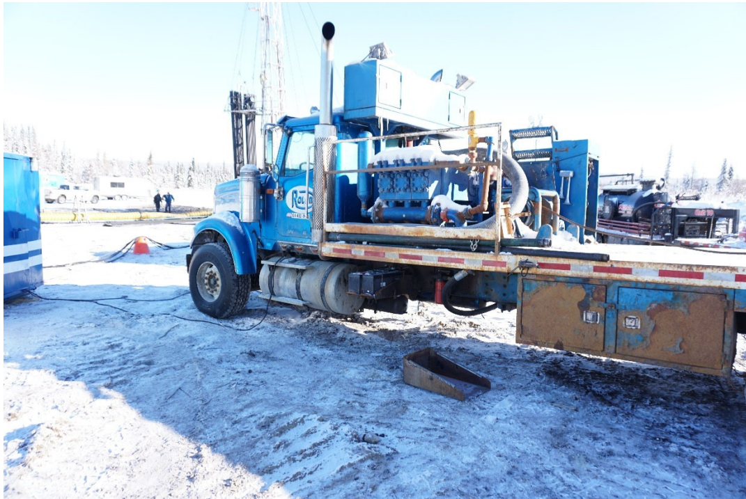
PHOTO #12: This piece of equipment required a drip tray placed underneath which was used for transporting the Accumulator shack.
