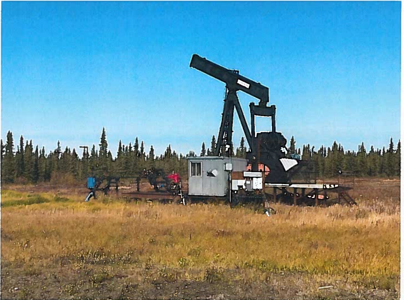
Photo # 1: Well Site - No wind indicator at well site. Wind indicator should be installed on well site.
